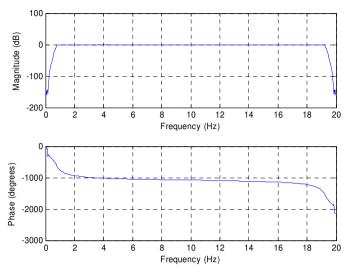
Fig.8. Spectrum response of the band-pass filter
