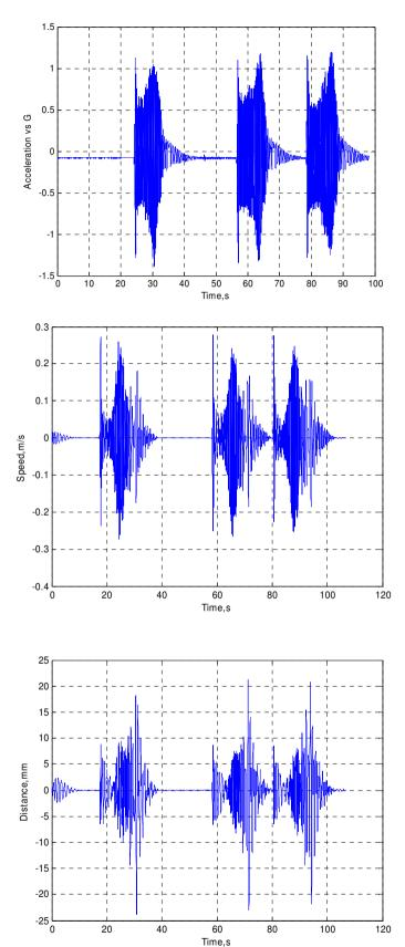
Fig.9. Measured stand acceleration and calculated speed and displacement after band-pass filter respectively
