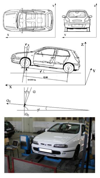
Fig. 2. Vehicle situation on the vibration stand
