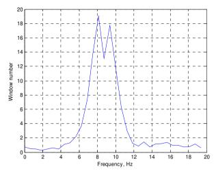
Fig. 6. Resonance frequencies of left and right dampers
