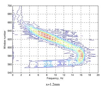
Fig.11. Spectrum response of the stand vibration depending on the clearance between the lower control arm of the suspension and the lower ball joint of the "candle"
