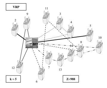
Figure 5 - Clarke and Wright's algorithm final solution for the VRP
