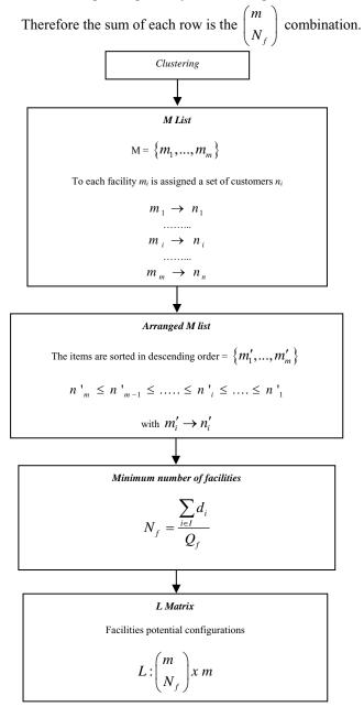
Figure 1 - LAP solving procedure
