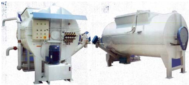
Fig. 1 the lime slaking and delivery machine under control
