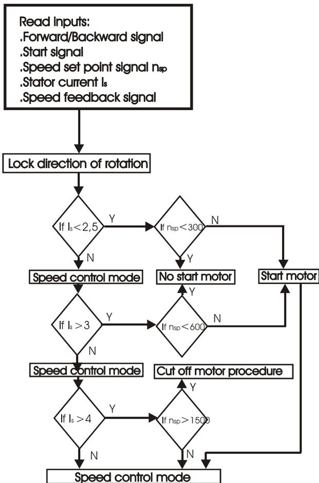
Fig. 5. Flowchart of monitor and protection Software
