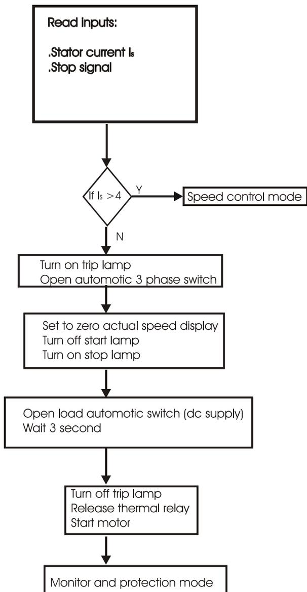
Fig. 6. Flowchart of cutoff/restart motor software
