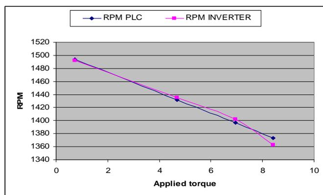
Fig. 7. Experimental speed torque characteristics with PLC and inverter
