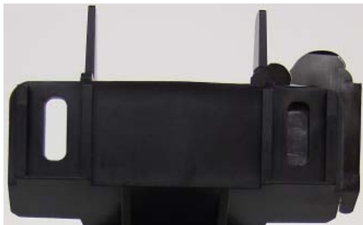
Fig. 21 Defects on part – flashes
