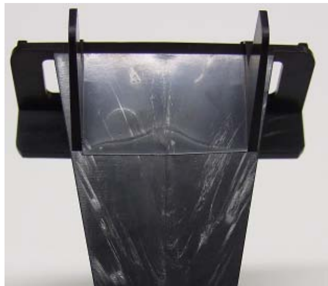
Fig. 25 Defects on part – color streak marks
