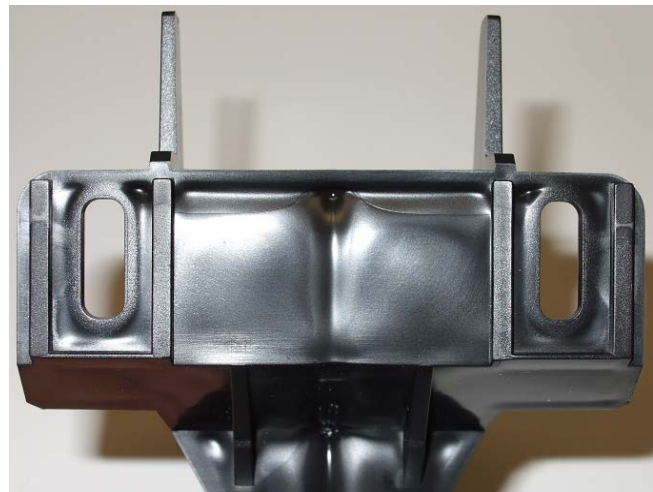
Fig. 24 Defects on part – sin marks
