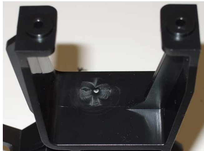
Fig. 23 Defects on part – hesitation marks
