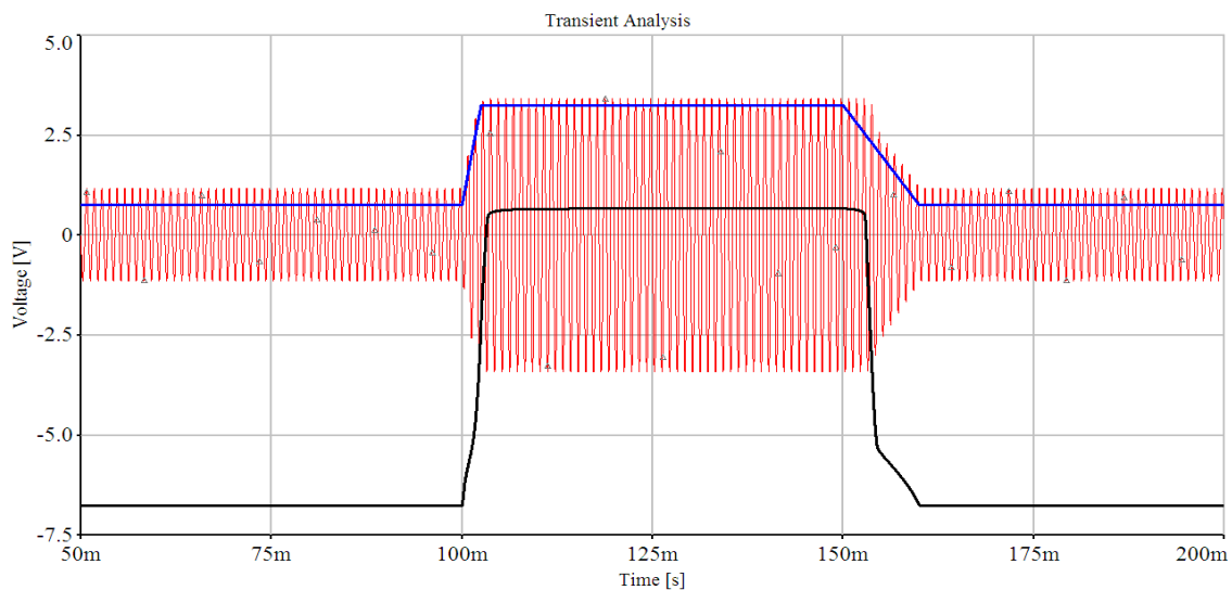
Fig. 14 VCA response to the input control voltage (fast sweep)
