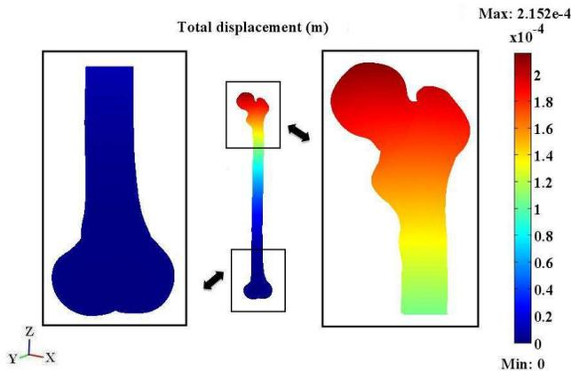
Fig. 7. Total displacement of the loading approximates the peak gait load for a 200 kg person during horizontal walking.
