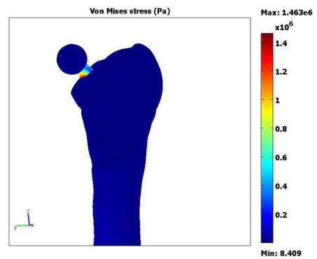
Fig. 18. Von Mises stress for a 70 kg person during normal walking.
