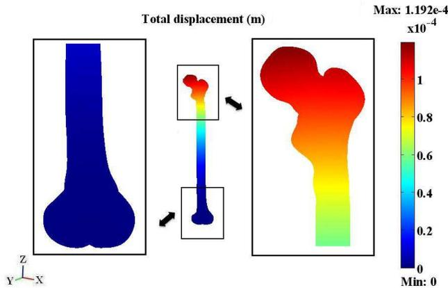
Fig. 6. Total displacement of the loading approximates the peak gait load for a 100 kg person during horizontal walking.
