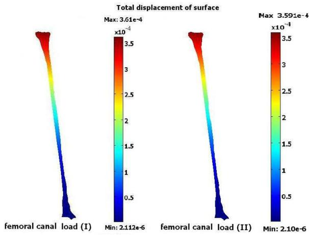
Fig. 14. Surface plot of the total displacement of femoral canal at load (I) and load (II).
