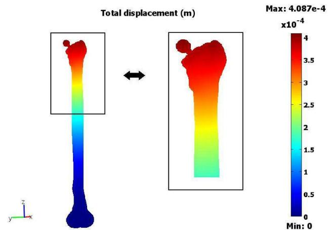
Fig. 12. Total displacement at a 70 kg person during normal walking.
