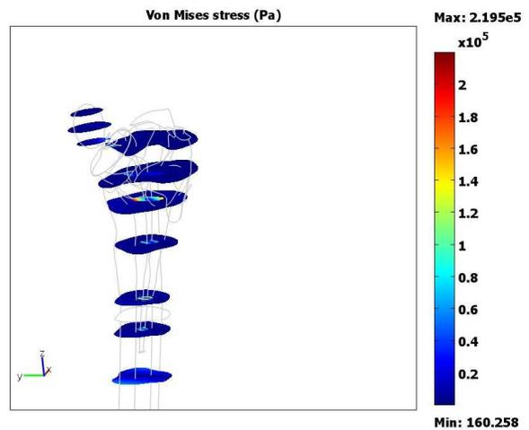
Fig. 19. Von Mises stress for a 70 kg person during normal walking.
