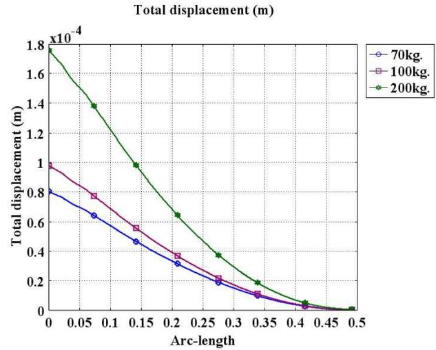
Fig. 8. Profile of total displacement along the axial of femur bone where the solid-circled line corresponds to the load of 70 kg, the solid-squared line corresponds to the load of 100 kg, and the solid-starred line corresponds to the load of 200 kg.
