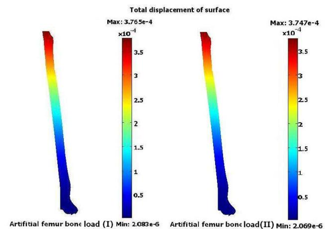
Fig. 13. Surface plot of the total displacement of artificial femur bone at load (I) and load (II).
