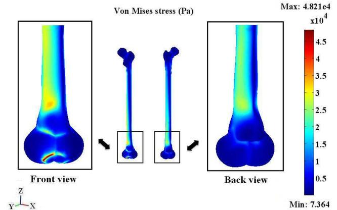
Fig. 9. Von Mises stress of the loading approximates the peak gait load for a 70 kg person during horizontal walking.
