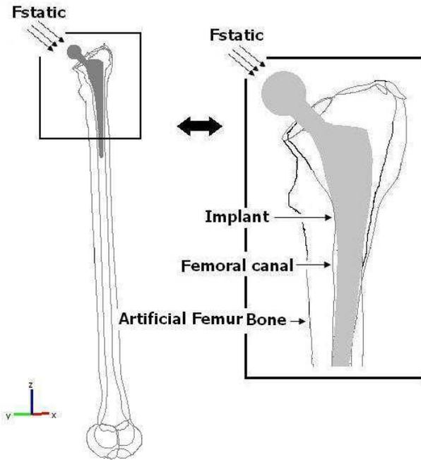
Fig. 2. The artificial femur bone geometry consists femoral canal bone and implant. Forces on the head implant.
