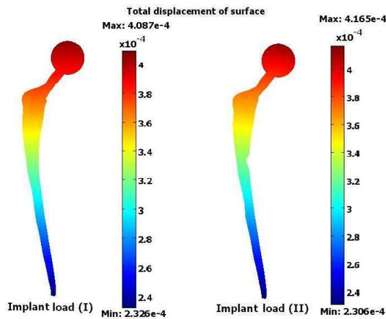
Fig. 15. Surface plot of the total displacement of implant at load (I) and load (II).
