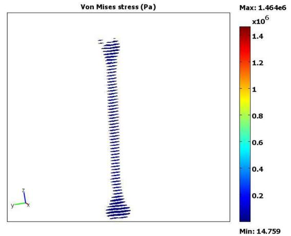
Fig. 17. Von Mises stress for a 70 kg person during normal walking.
