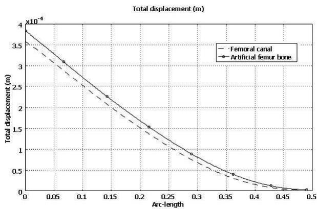
Fig. 16. Profile of the total displacement along the axial of artificial femur bone where the solid-circled line, and the dashed line corresponds to the femoral canal for a 70 kg person during normal walking.
