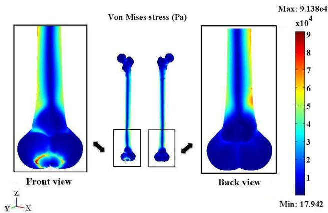
Fig. 11. Von Mises stress of the loading approximates the peak gait load for a 200 kg person during horizontal walking.
