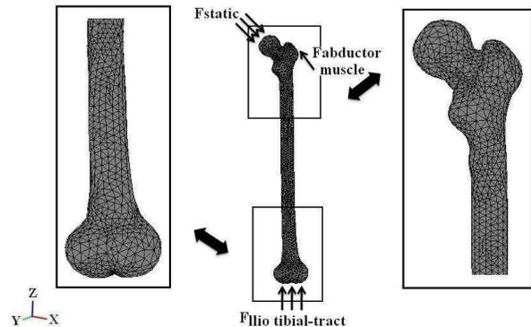
Fig. 1. Three-dimensional geometry of fumer bone and its finite element mesh.
