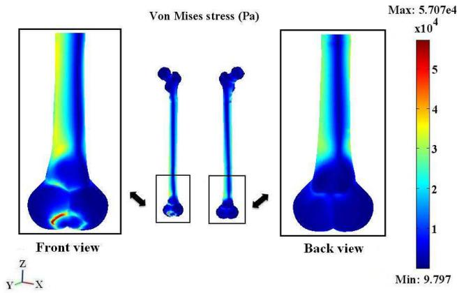
Fig. 10. Von Mises stress of the loading approximates the peak gait load for a 100 kg person during horizontal walking.
