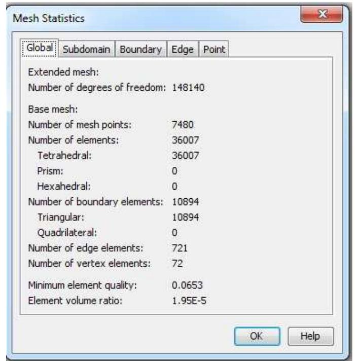
Fig. 4. Mesh statistic of the artificial femur bone geometry.
