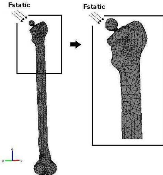
Fig. 3. Mesh of the artificial femur bone geometry consists of 36,007 tetrahedral elements and 148,140 degrees of freedom. Forces on the head implant.
