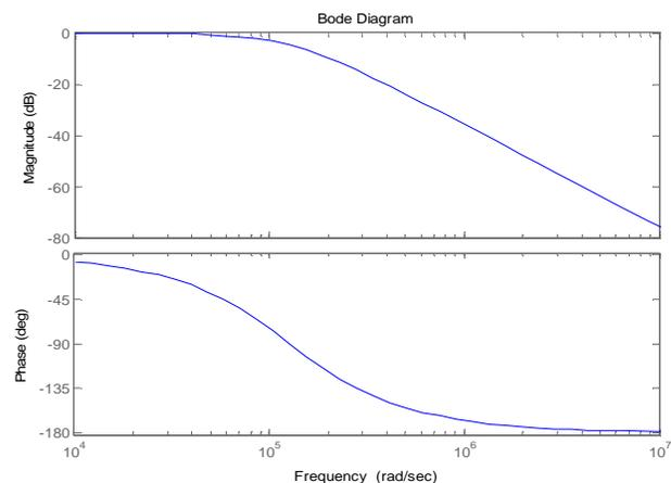
Fig. 8 Filter Bode frequency response simulation.
