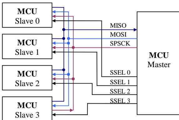
Fig. 9 Serial peripheral interface operation.
