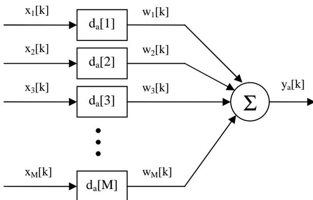
Fig. 1 Delay and sum beamformer operation.
