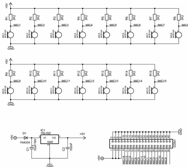
Fig. 5 Microphone array board schematic.
