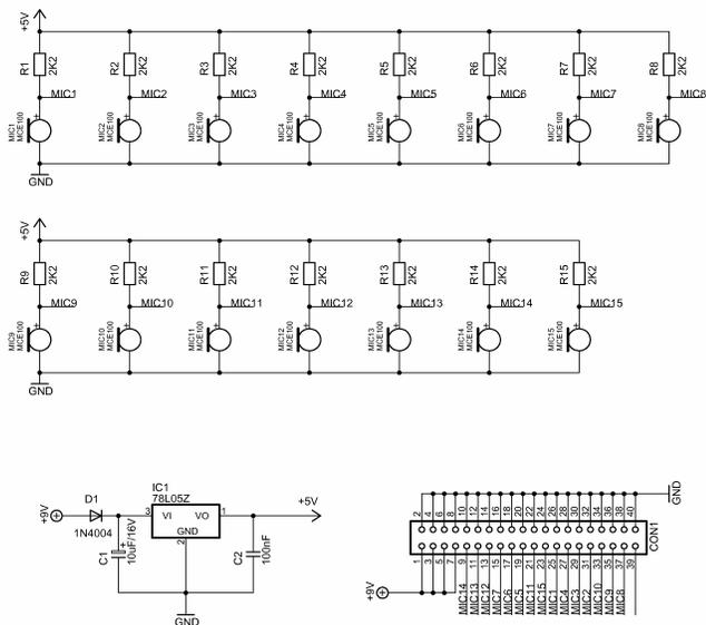
Fig. 5 Microphone array board schematic.
