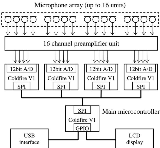
Fig. 3 Localization system architecture.
