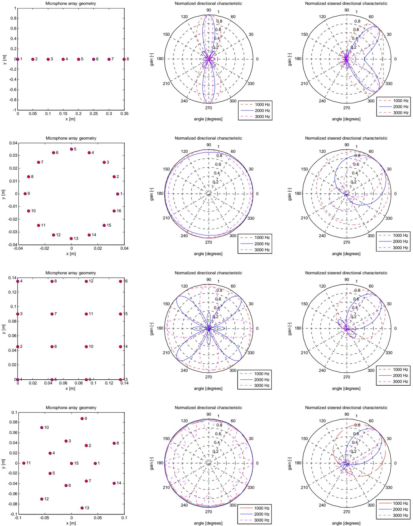
Fig. 4 Simulated directional characteristics of different microphone array geometrical configuration.
