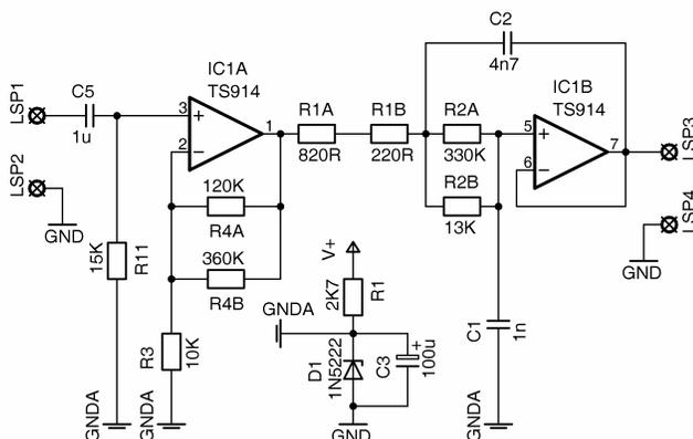
Fig. 7 Microphone array preamplifier schematic for one channel.
