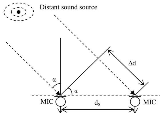
Fig. 2 Sound wave impacting pair of sensors.
