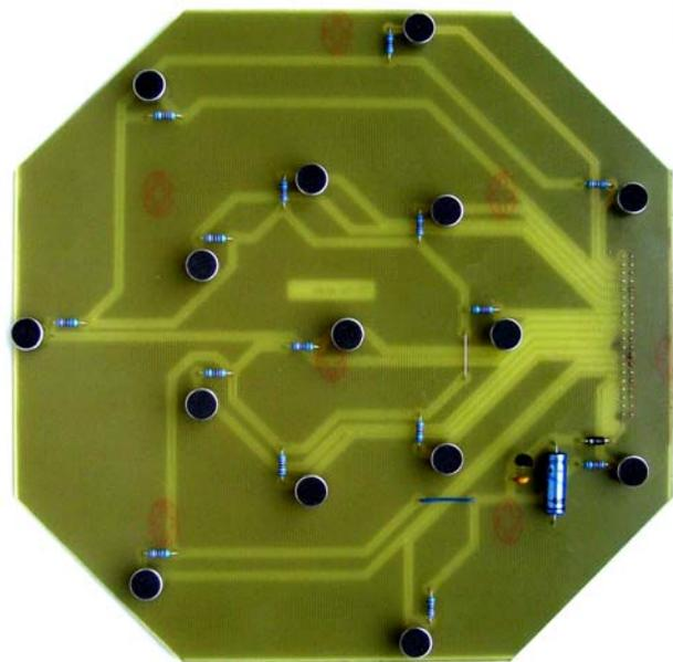
Fig. 6 Photograph of the completed microphone array board.
