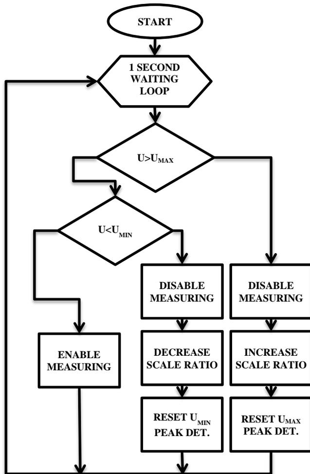
Fig. 9 – Autonomous input buffer and prescaler operation flowchart
