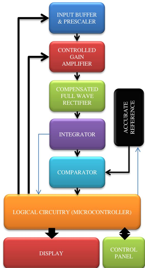
Fig. 8 - Block diagram of the suggested voltmeter disposition
