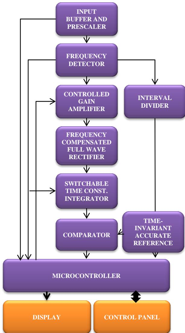
Fig. 11 – Optimized configuration of the suggested voltmeter disposition
