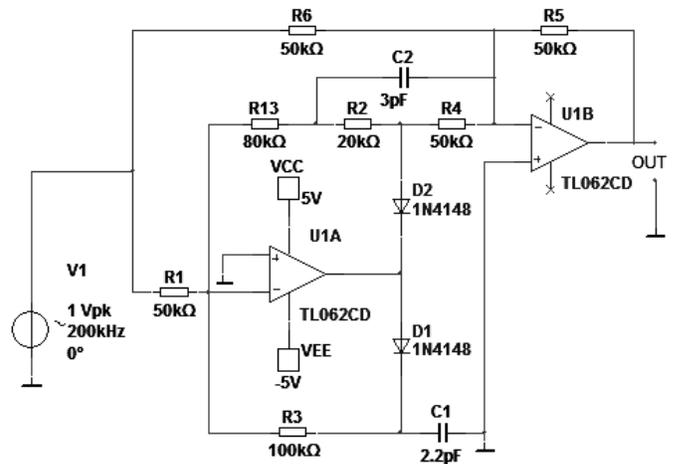
Fig. 4 - Modified full wave rectifier with frequency compensation
