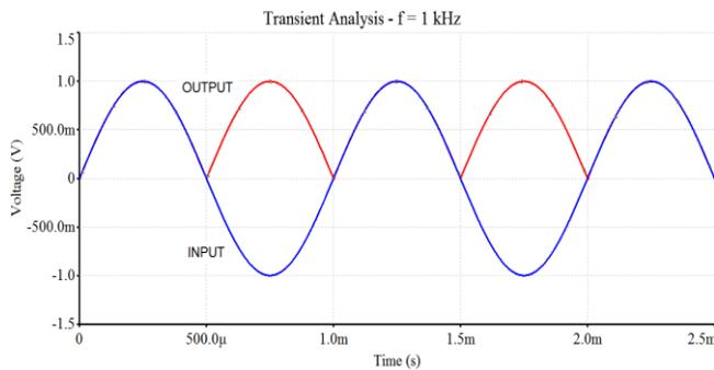
Fig. 2 - Full wave rectifier from Fig. 1 input and output at f = 1 kHz (simulation)
