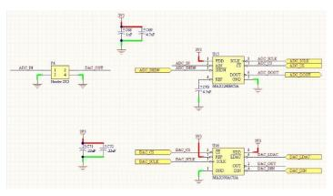
Fig. 11 ADC/DAC schematic diagram
