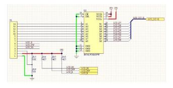
Fig. 13 Liquid Crystal Display schematic diagram
