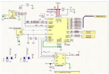
Fig. 8 USB schematic diagram using a transceiver chip
