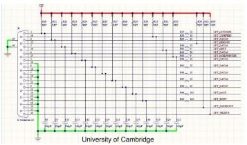
Fig. 9 Parallel Port Pin Assignment
