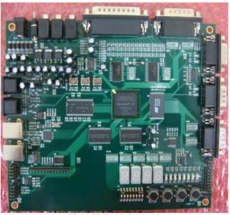
Fig. 2 FPGA Motherboard
