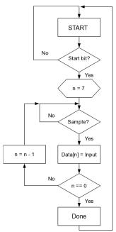
Fig. 6 UART Receive Process
