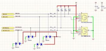
Fig. 7 PS/2 Ports Schematic Diagram
