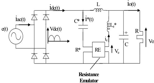
Fig. 5. Modifying the passive PFC, by means of a resistance emulator circuit
