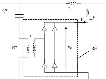
Fig. 6. The proposed resistance emulator circuit
