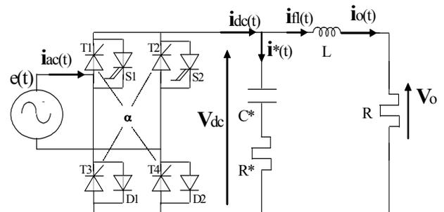
Fig. 9. Modified single-phase thyristor-based rectifier circuit, with passive PF correction
