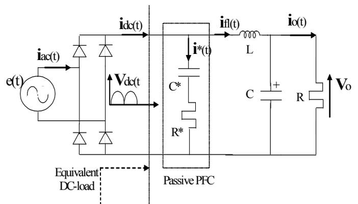
Fig. 3. Single-phase diode bridge rectifier scheme with L-C DC-filter and the proposed PFC
