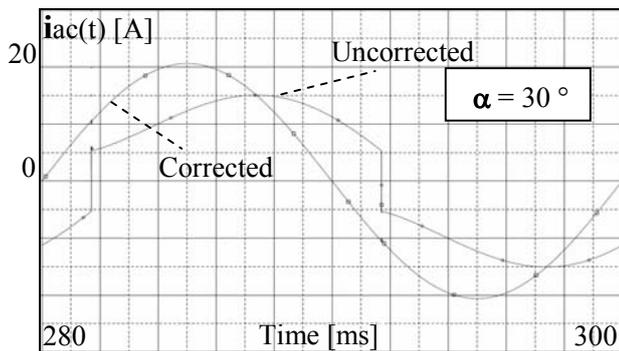
Fig. 11. AC-side rectifier current waveforms without and with the proposed PFC, for different values of  $\alpha$ .
