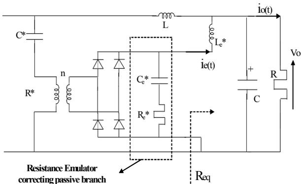
Fig. 7. The proposed resistance emulator, with its passive correction
