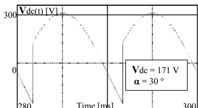
Fig. 12. DC-side rectifier voltage waveforms without and with the proposed PFC, for different values of  $\alpha$ .
