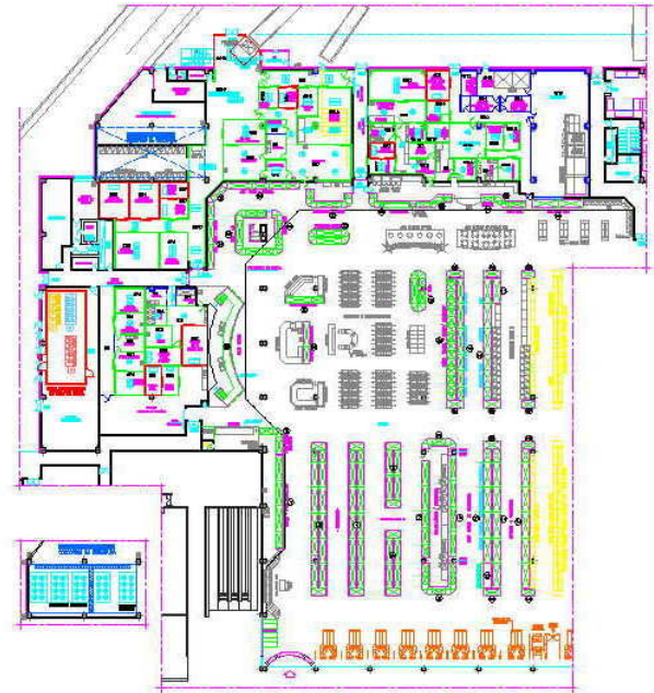
Figure 11 – Jumbo de Almada layout with refrigeration equipment
