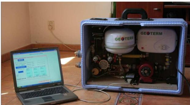
Fig. 5 Testing equipment GEOTERM PDC
