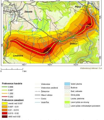
Fig. 4 Scaled frequencies of partial areas exposure in case of transport of 20 tons of ammonia upon introduction of local situation modification
