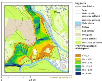
Fig. 5 Standardized impact frequencies for partial areas upon leakage of 30m of liquid
