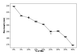
Fig. 21 Influence of the flow length on filler amount (Grinded plate)
