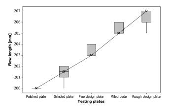
Fig. 15 Influence of the flow length on surface quality (20% glass fibers)
