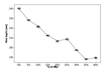
Fig. 24 Influence of the flow length on filler amount (Rough design plate)
