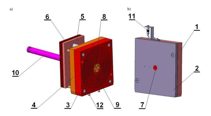
Fig. 3 Shaping part of the injection mold a) left side, b) right side
