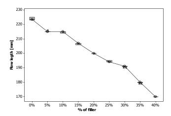
Fig. 20 Influence of the flow length on filler amount (Polished plate)
