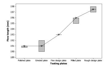
Fig. 17 Influence of the flow length on surface quality (30% glass fibers)
