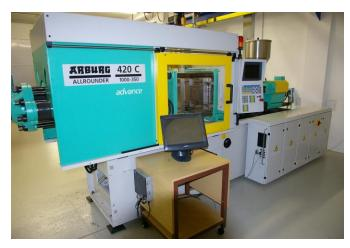
Fig. 8 Injection molding machine ARBURG Allrounder 420C
