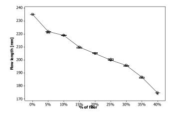
Fig. 23 Influence of the flow length on filler amount (Milled plate)
