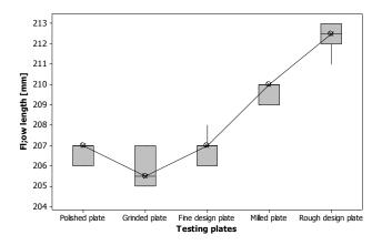
Fig. 14 Influence of the flow length on surface quality (15% glass fibers)
