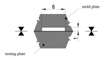
Fig. 4 Cross section of mold cavity
