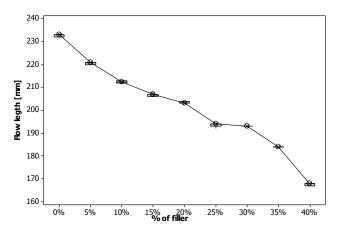
Fig. 22 Influence of the flow length on filler amount (Fine design plate)
