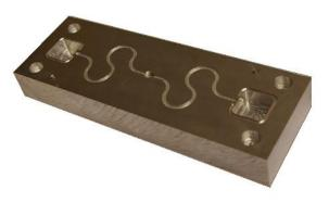
Fig.5 Model of upper part of mold
