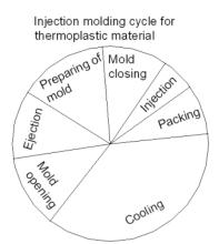
Fig.1 Thermoplastic injection molding cycle
