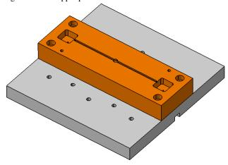
Fig.6 Universal frame with cavity plate (lower part)
