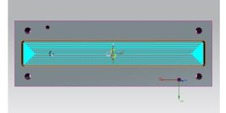
Fig.12 Roughening space for sensors
