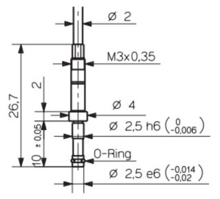
Fig.14 Dimension of sensor
