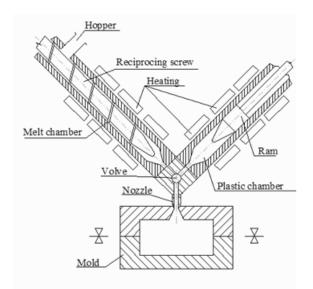
Fig.19 Schema of REP V27/Y125 machine
