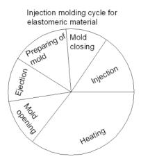
Fig.2 Elastomeric injection molding cycle
