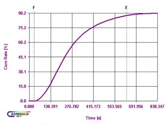
Fig.21 Sample of Cure curve Cadmould rubber software for this issue
