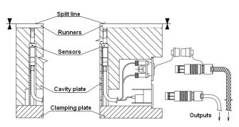
Fig.17 Situation sensors in mold
