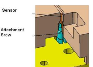
Fig.15 Attached sensor in runner
