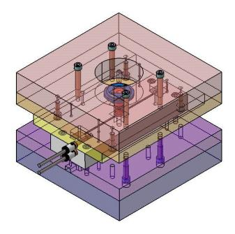
Fig.4 Model of assembled mold
