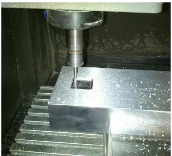
Fig.25 Illustration of manufacturing of cavity
