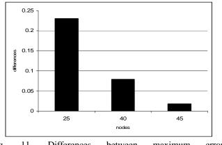
Fig. 11. Differences between maximum errors (|ERR - ERRNUM|), for different number of nodes:
