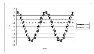
Fig.4 Exact and numerical values of *cp* for 20 nodes on the boundary.
