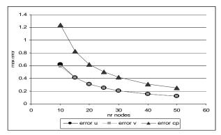
Fig.6 Influence of mesh refinement on errors.
