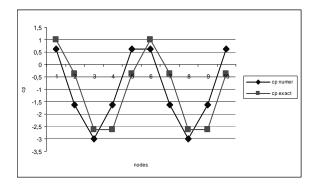
Fig.3 Exact and numerical values of *cp* for 10 nodes on the boundary.
