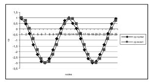
Fig.5 Exact and numerical values of *cp* for 25 nodes on the boundary.
