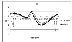
Fig.8. Exact and numerical local pressure coefficient for 40 nodes on the boundary.
