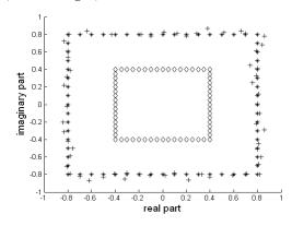
Fig. 6 inversion results for similarity transformation showing target outputs by *diamonds* expected inputs by *stars* actual inputs obtained from inversion by plus signs
