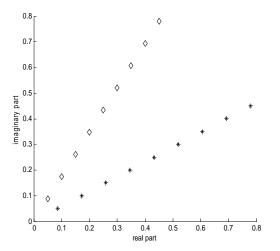
Fig. 7 training data for rotational transform in complex plane: *stars* showing inputs and *diamond* symbols showing corresponding outputs
