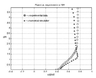
Figure 5c Mean velocity profile x = 10H
