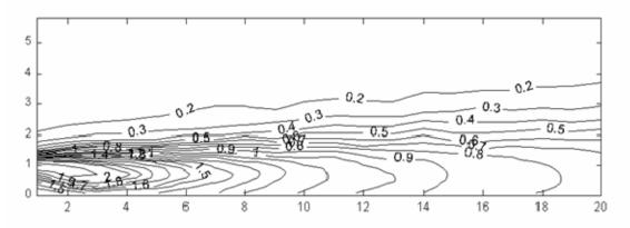
Figure 7. The profiles of the velocity fluctuations Urms (experimental data)
