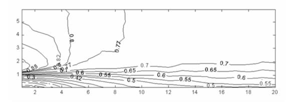
Figure 6b The profiles of the axial mean velocity Ux (experimental data)
