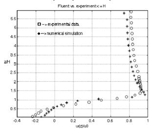
Figure 5a Mean velocity profile x = H
