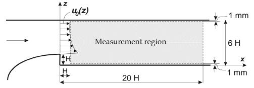
Figure 3. The measurements domain (H=10mm)
