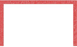
Fig.13. unstructured mesh applied for GFVM solver
