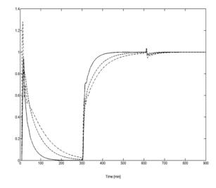
Fig.5 Closed-loop response to sequential step changes in set-point for OR column
