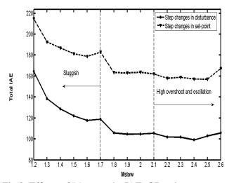
Fig.2 Effects of Ms<sub>low</sub> on the IAE: OR column.
