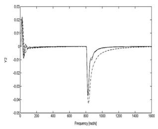
Fig.4 Closed-loop response to sequential step changes in disturbance for WW column
