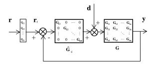
Fig.1 Block diagram for the multi-loop control system.
