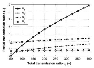
Fig 3: Partial ratios versus the total transmission ratio
