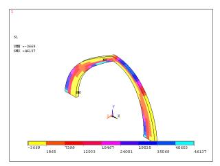
Fig X: Four centered pointed arch modeling by ansys
