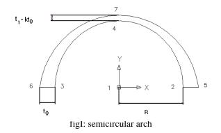
In arch modeling, the tolerance increases because the thickness decreases from base to top. We should remember that in modeled arch, the thickness decrease from base (t0) to top (t1) linearly. Also, arch thickness in direction of length axis is 20 cm. The motion of support nodes is zero, and dynamic force has no effect on them. Also, brick masonry is made by brick and mortar as homogenous material (table I). The efficient factors in inelastic nonlinear analysis show in (table II). [4,7,12]
