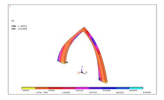
Fig III: Catenary arch modeling by ansys
