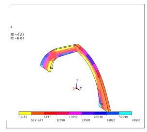
Fig VII: Catenary arch modeling by ansys
