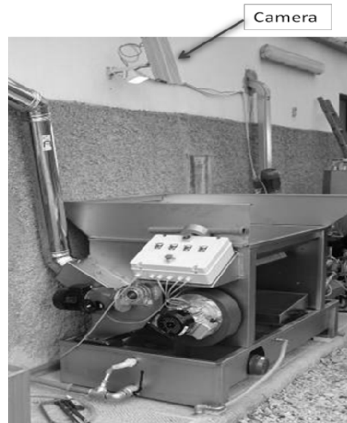
Fig. 3 – Positioning of the CMOS camera.
