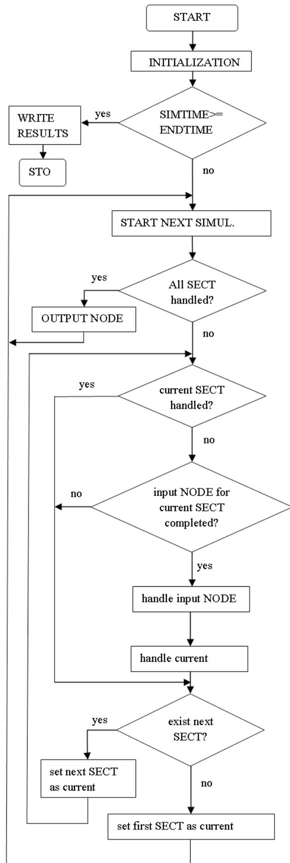
Fig. 2 Block diagram for class SIMULATOR
