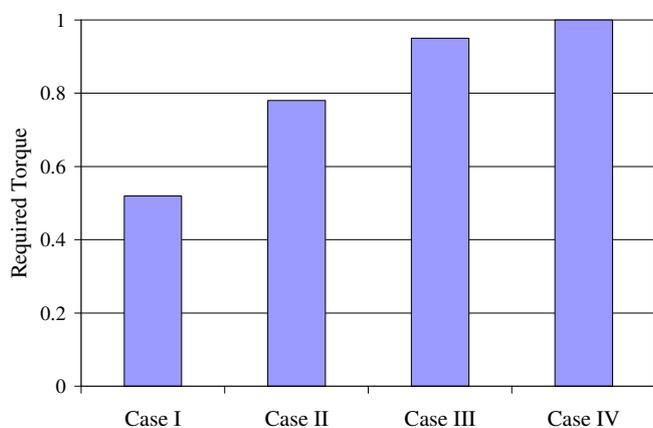
Fig. 7. Required torque to run the platforms in the software.
