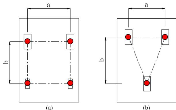
Fig. 2. Stability area for two mechanisms having the same dimensions.
