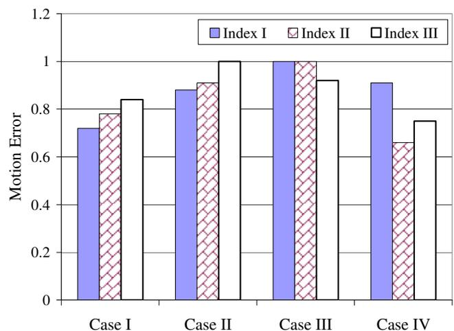
Fig. 5. Normalized values of position error along paths defined to evaluate performance along straight line (index I), curvature line (index II), and multiple line (index III).
