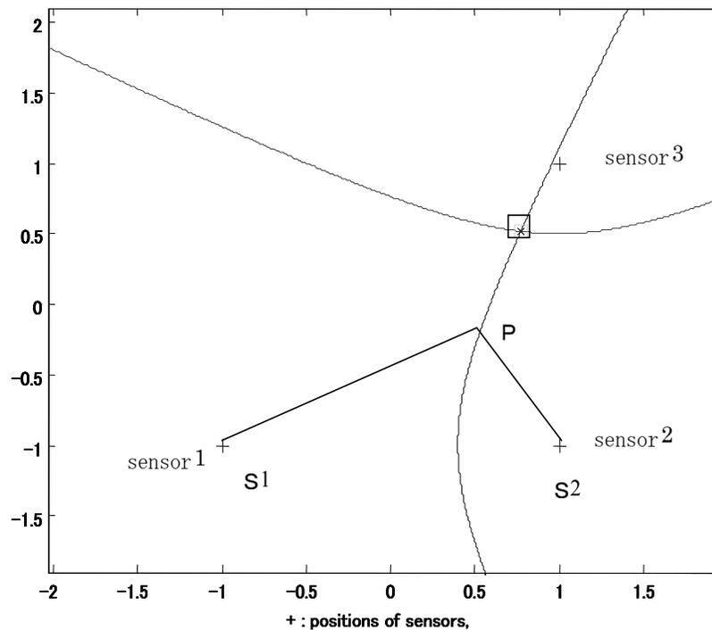
Fig. 3 Principle of the Hyperbolic Method.
