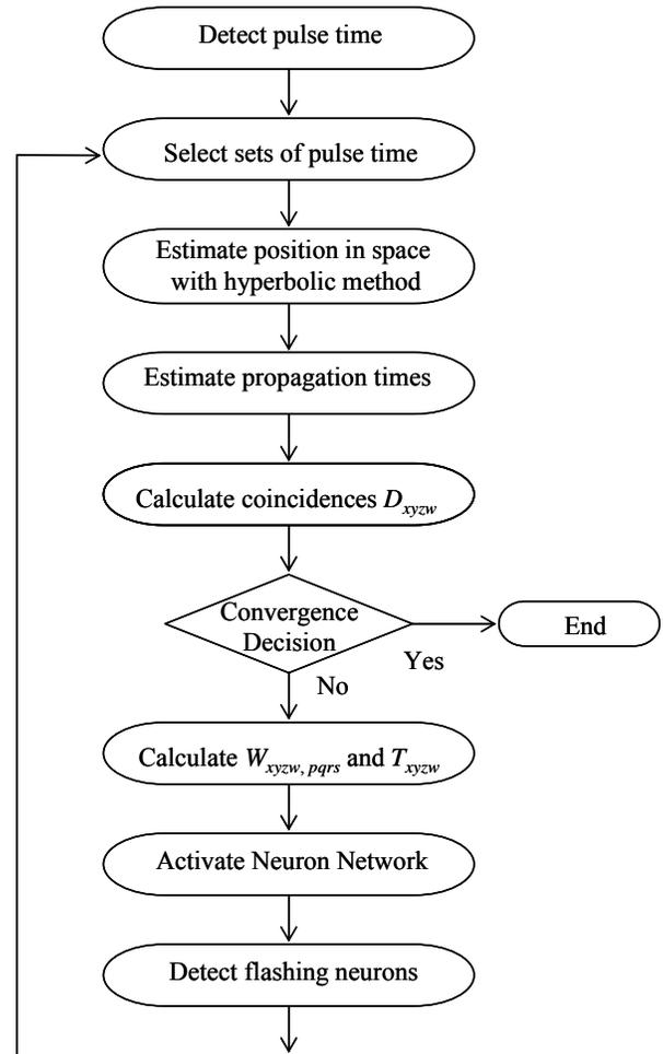
Fig. A1 Calculation Flow.
