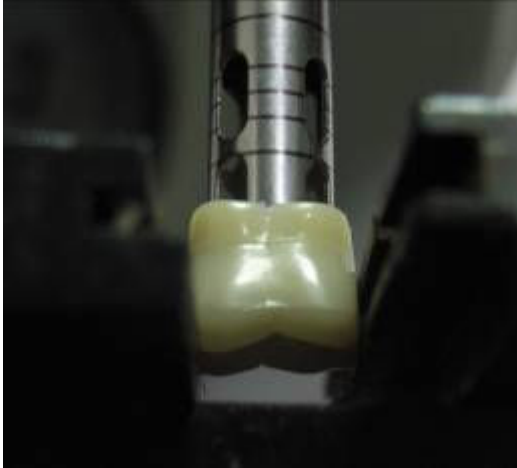
Fig.6. Vestibulo-occlusal aspect of the cylinder milled with the trepan bur inside the acrylic tooth
