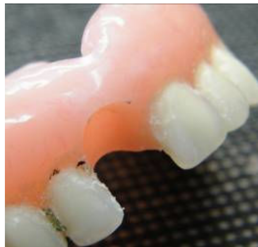
Fig.2. Acrylic tooth detached from denture base resin: detail.
