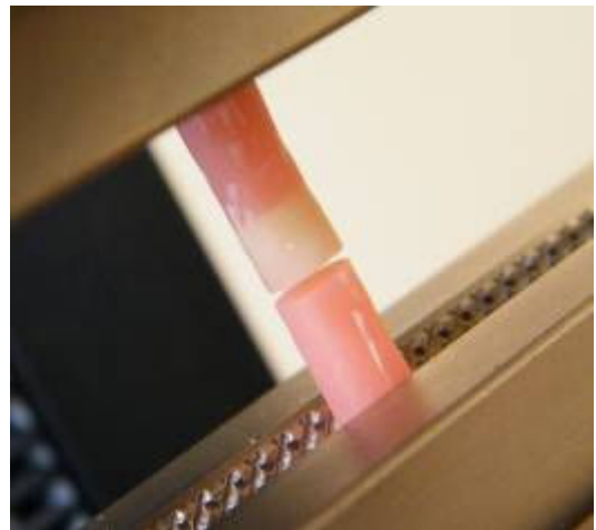
Fig.17. Detaile of the tensile test sample after the adhesive fracture
