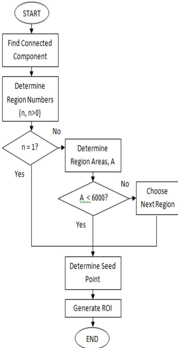
Fig. 7 Algorithm for seed point detection
