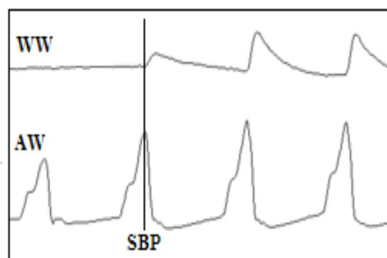
Figure 10. Wrist waveforms (WW) and arm waveforms (AW) obtained simultaneously. Systolic pressure (SBP) is the point of WW appearance.
