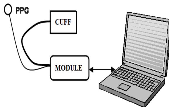
Figure 2. The system for acquisition of wrist-cuff and finger PPG waveforms.
