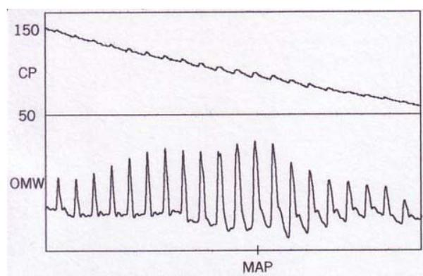
Figure 1. Cuff pressures (CP) and oscillometric waveforms (OMW) acquired during gradual cuff deflation.
