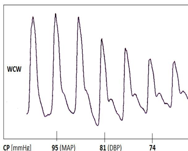
Figure 5. Wrist cuff waveforms (WCW) obtained at cuff pressures near DBP.
