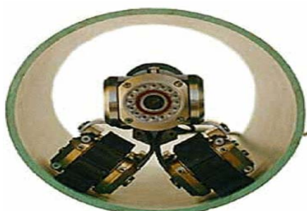
Fig. 5: Example of robot used in pipe inspection.
