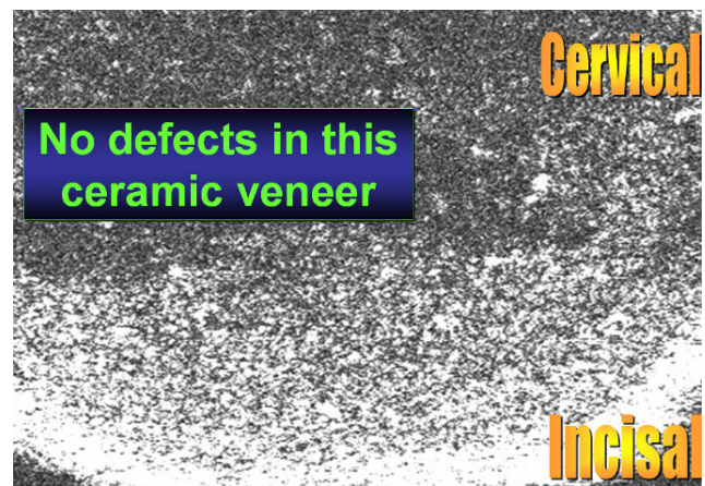
Fig. 14. En Face OCT investigation of ceramic veneer sample nr.7. Slice 36 from 110 stuck images with 18 degree scanning.
