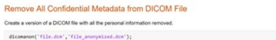
Fig. 1 Screenshot of Matlab's code creating the anonymized copy of file.dcm which is named file_anonymized.dcm
