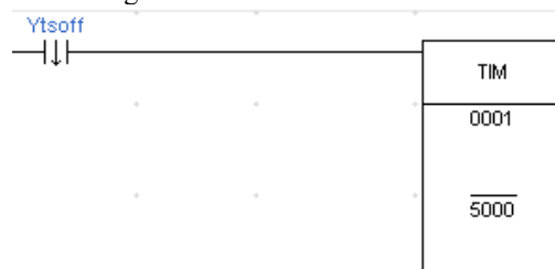
Fig. 13. Ladder diagram for timer control (TIM)
