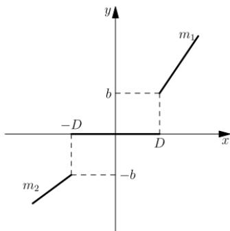
Fig. 3 Discontinuous nonlinear characteristic
