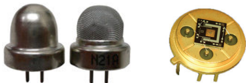
Fig.13 Design of sensors of measurement of gas mixture according to thermal conductivity and picture of its MEMS technology (NEMOTO).
