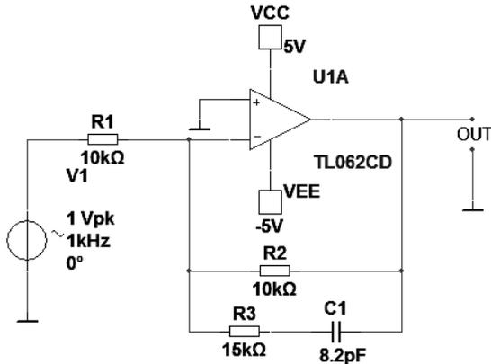
Fig. 6 - Simple preamplifier for additional frequency compensation
