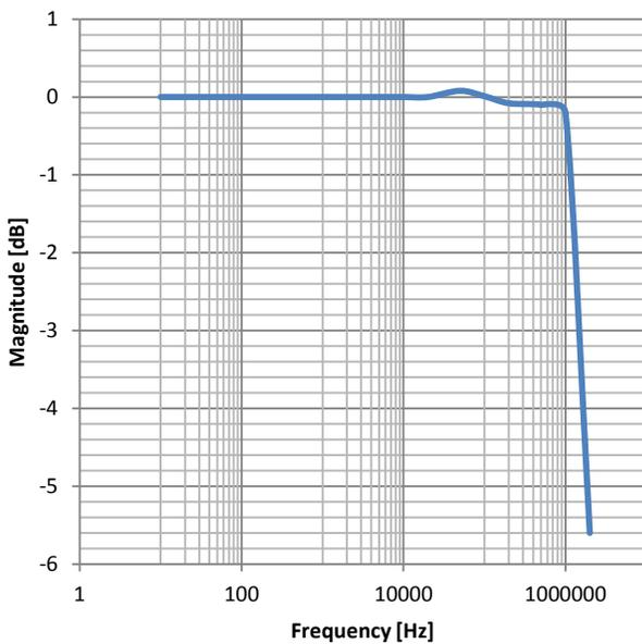
Fig. 7 - Frequency response of the well-compensated full wave rectifier from Fig. 4.
