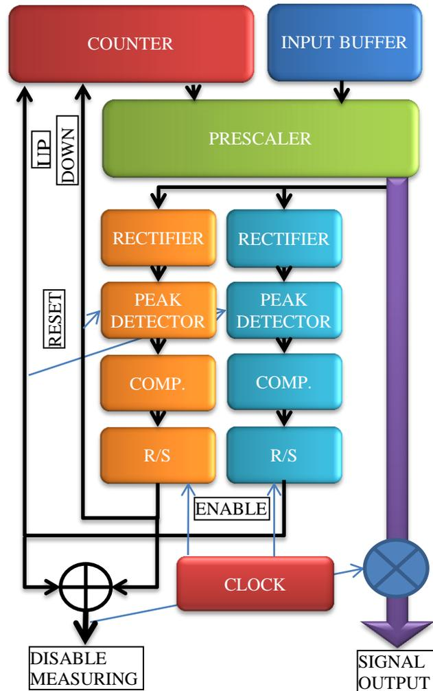
Fig. 10 – Block diagram of autonomous input buffer and prescaler constructed with the aid of logical gates
