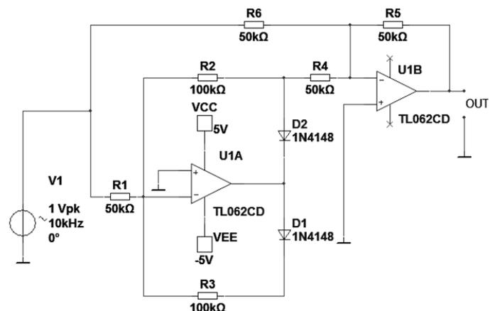
Fig. 1 – Simple full-wave rectifier simulation schematics
