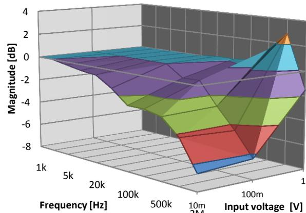
Fig. 5. - Attenuation of the frequency compensated rectifier at different voltage levels and different frequencies
