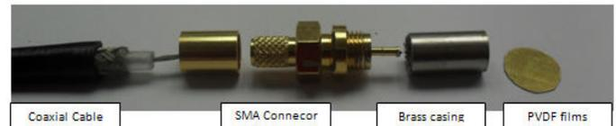
Fig. 10 PVDF sensor with SMA connector
