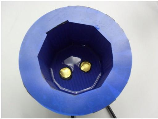
Fig. 11 Complete design of PVDF sensor water-tank casing
