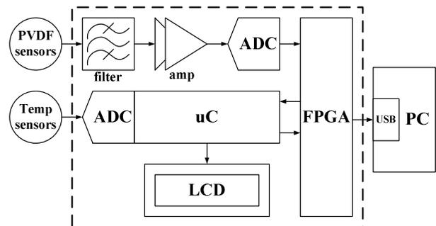
Fig. 14 Block diagram of ultrasound power meter
