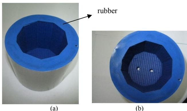
Fig. 9 Rubber inside the casing: top view (a), side view (b)
