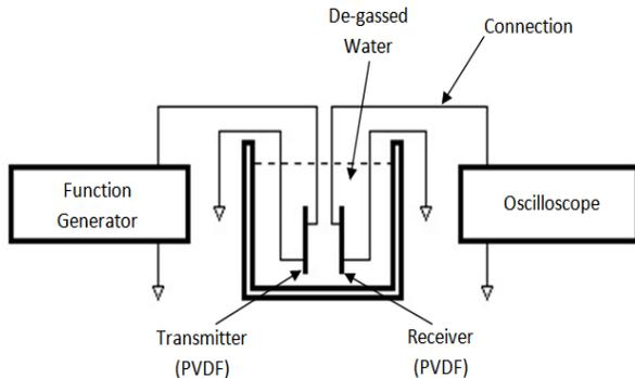
Fig. 2 Diagram of PVDF experiment setup
