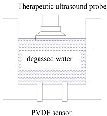
Fig. 12 Water-tank implementation setup
