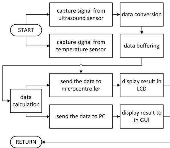
Fig. 15 System design of the ultrasound processing unit
