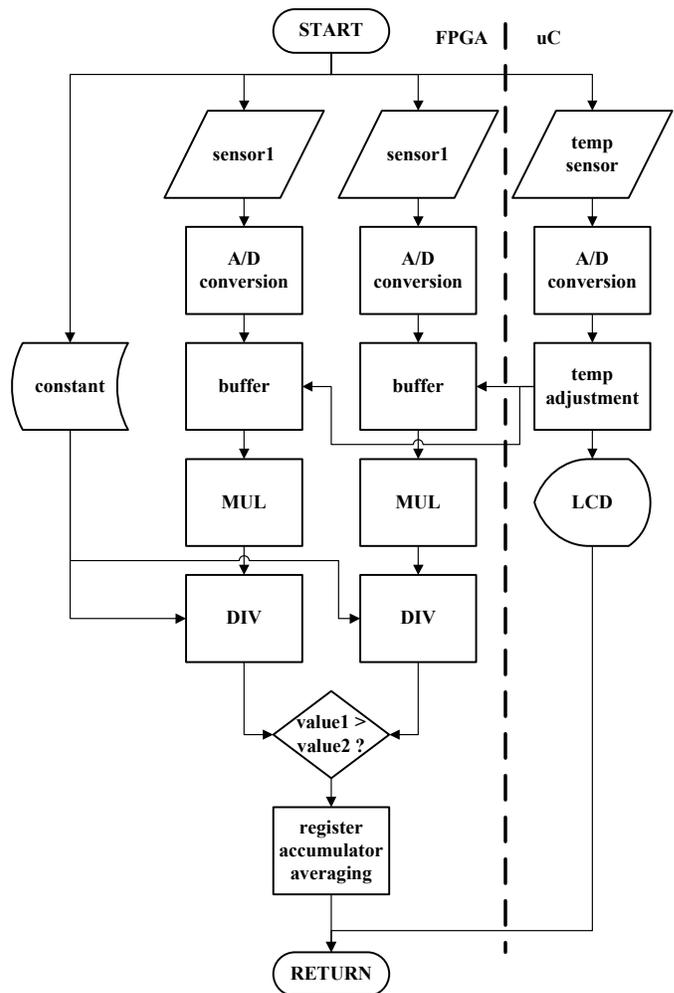
Fig. 16 Algorithm of ultrasound intensity calculation
