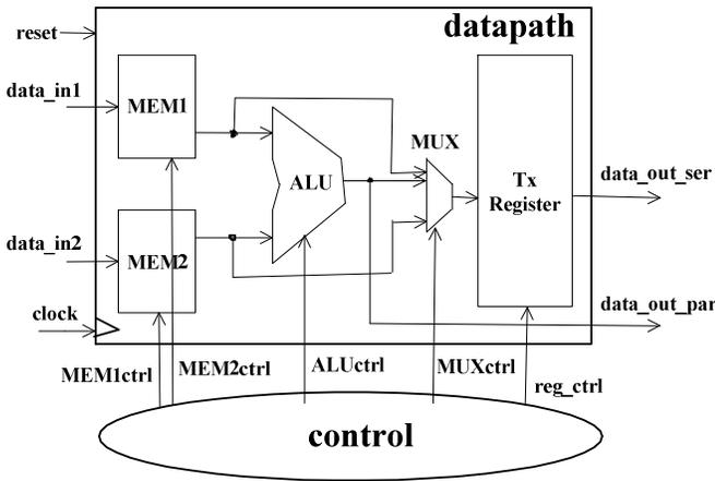
Fig. 17 RTL block diagram of ultrasound processing unit
