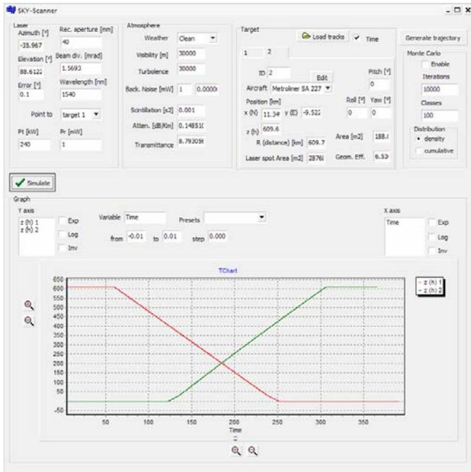
Fig. 11 Landing A321 colliding with taking off Metroliner. represented with the green line. We show the height of both airplanes vs. time.
