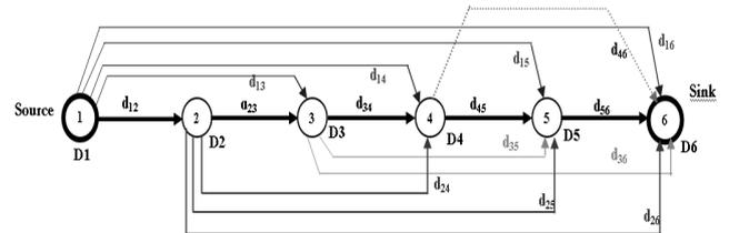
Fig. 1 Delays involved by candidate positions for buffer insertion
