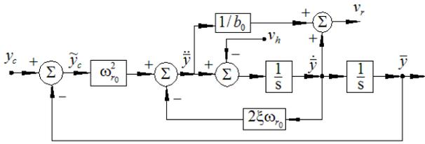
Fig. 7. The block diagram of the reference model
