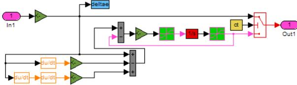
Fig. 11. Matlab/Simulink model of "Forming subsystem for vector deltae (r=2)"
