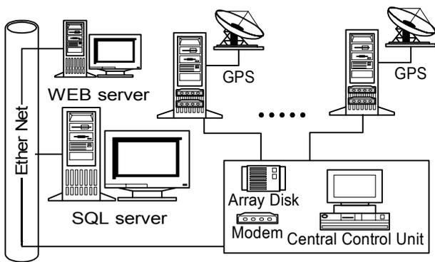
Fig. 5. Schematic arrangement of the WAMS hardware.
