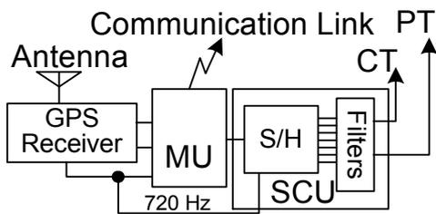
Fig. 6. Block diagram of synchronous phasor measurement system.
