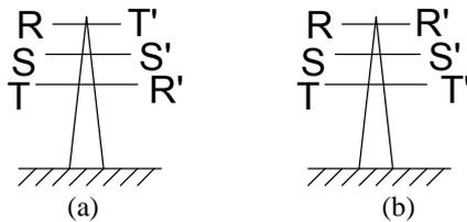
Fig. 2. The conductor space arrangement (a) non-perfectly symmetrical RST-T'S'R', (b) asymmetrical RST-R'S'T'.
