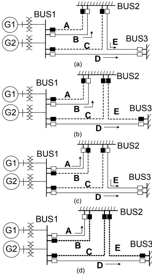
Fig. 9. N-2 conditions at different towers with short distance lines being opened (a) Case 2-2A (circuits A and C being opened), (b) Case 2-2B (circuits A, C, and E being opened), (c) Case 2-4A (circuits B and C being opened), (d) Case 2-4B (circuits B, C, and E being opened)
