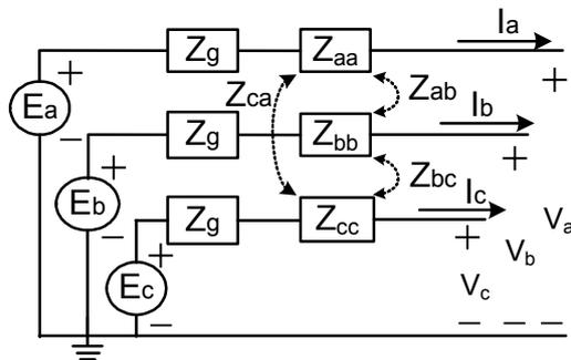
Fig. 3. Three-phase balanced source and untransposed transmission lines.
