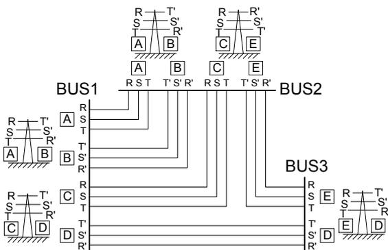
Fig. 8. Conductor arrangement of the transmission lines.
