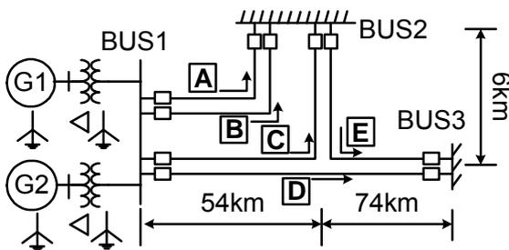
Fig. 7. One-line diagram of the 345-kV transmission system (arrow indicates current direction in the N-0 condition).
