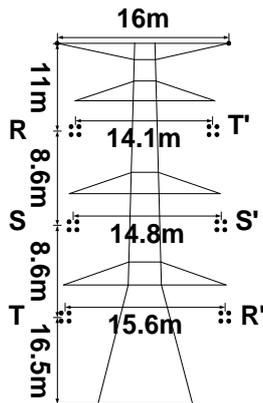
Fig. A1 Cross section of the 345-kV power line corridor.
