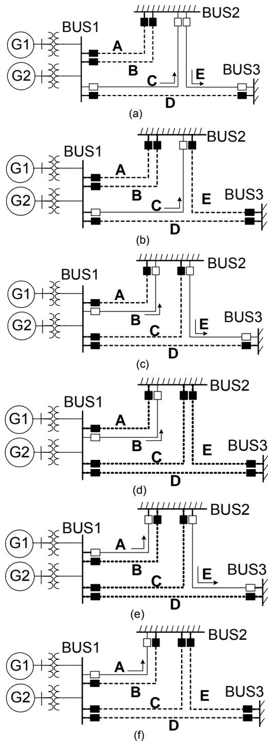
Fig. 11. N-3 conditions with long lines being opened (a) Case 3-2A (circuits A, B, and D being opened), (b) Case 3-2B (circuits A, B, D, and E being opened), (c) Case 3-3A (circuits A, C, and D being opened), (d) Case 3-3B (circuits A, C, D, and E being opened), (e) Case 3-4A (circuits B, C, and D being opened), (f) Case 3-4B (circuits B, C, D, and E being opened).
