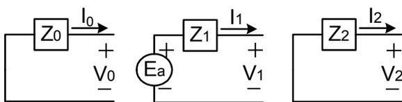
Fig. 4 Voltage sources in sequence networks.
