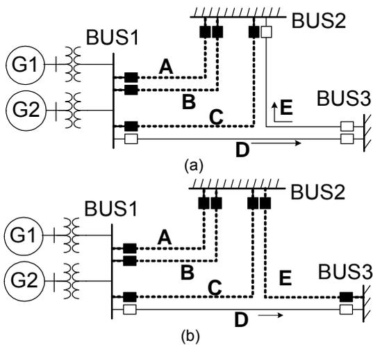
Fig. 10. N-3 conditions with short distance lines being opened (a) Case 3-1A (circuits A, B, and C being opened), (b) Case 3-1B (circuits A, B, C, and E being opened)
