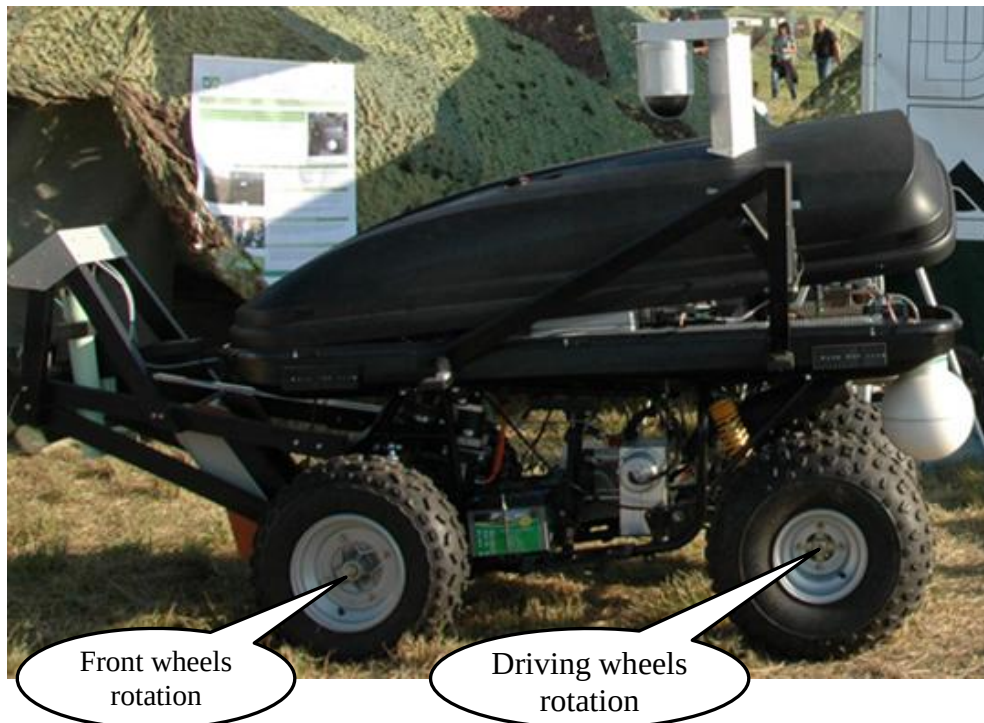
Fig. 13 Unmanned ground vehicle for radiation reconnaissance
