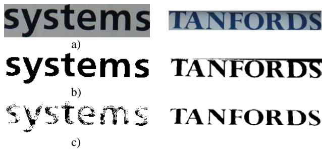
Fig. 8. Complementarity between intensity and saturation distance: original images (top), result of K-means with intensity distance (middle) and result of K-means with saturation distance (down)
