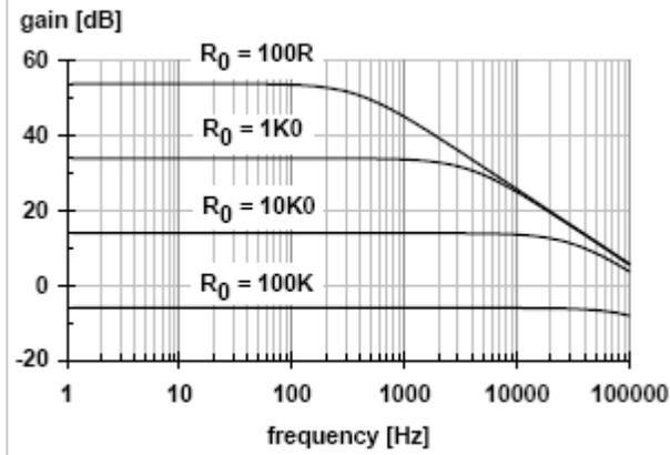
Fig. 18 frequency response at  $R_0 = 100 \Omega$  to  $100 \text{ k}\Omega$  operational amplifier MAA725
