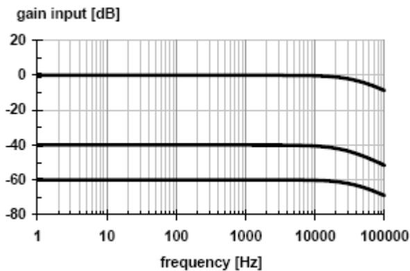
Fig. 6 frequency response the input units with operation amplifier MAA725
