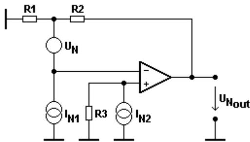
Fig. 11 operational amplifier noise model [9]
