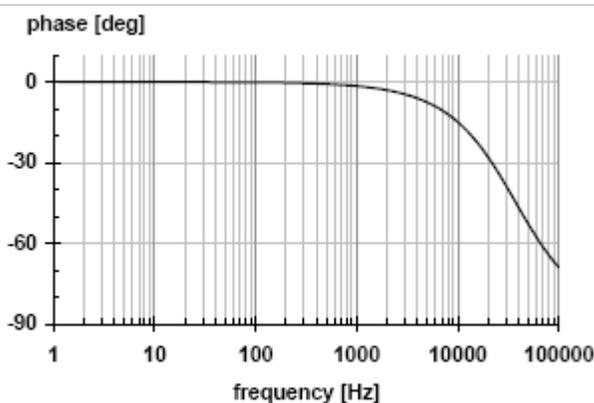
Fig. 7 phase response the input units with operation amplifier MAA725
