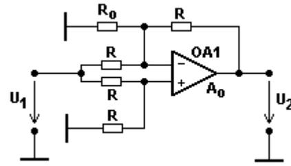
Fig. 17 scheme of the differential amplifier input unbalanced
