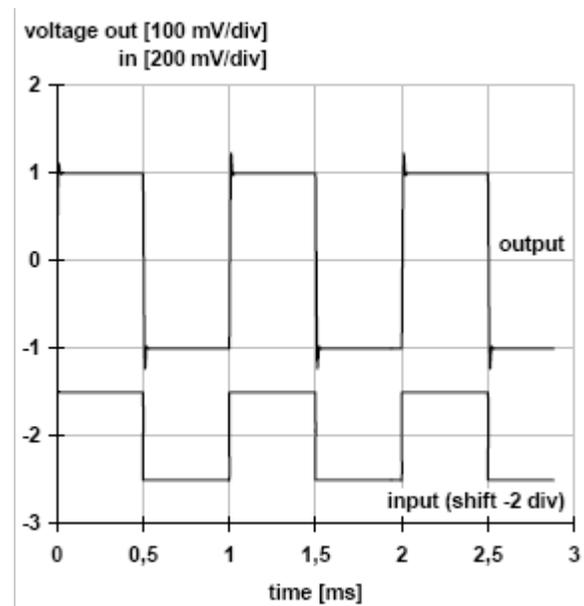
Fig. 8 response of input units on the input signal square 1 kHz
