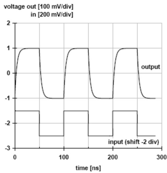
Fig. 9 response of input units on the input signal square 10 kHz
