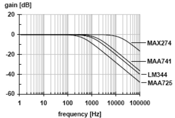
Fig. 14 frequency response at  $R_0 = 1$  k $\Omega$
