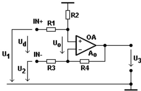
Fig. 16 scheme of the classics differential amplifier
