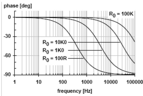
Fig. 19 phase response at  $R_0 = 100 \Omega$  to  $100 \text{ k}\Omega$  operational amplifier MAA725
