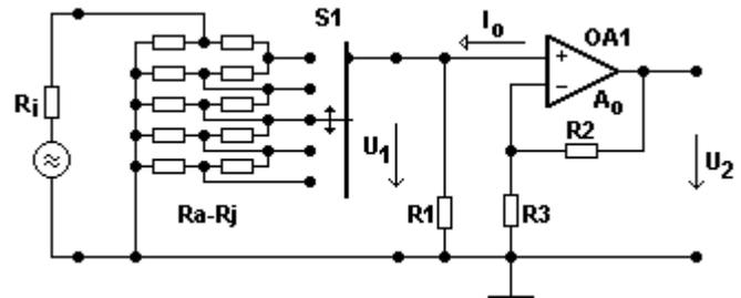
Fig. 3 the input amplifier chain with shock damping element
