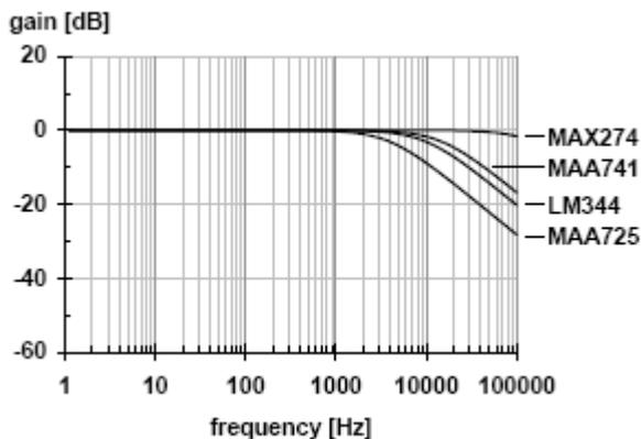
Fig. 12 frequency response at  $R_0 = 10$  k $\Omega$
