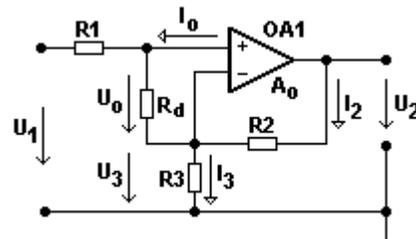
Fig. 4 principle diagram of an amplifier with high input resistance
