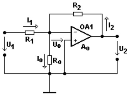
Fig. 10 scheme the amplifier with a resistor in a virtual zero
