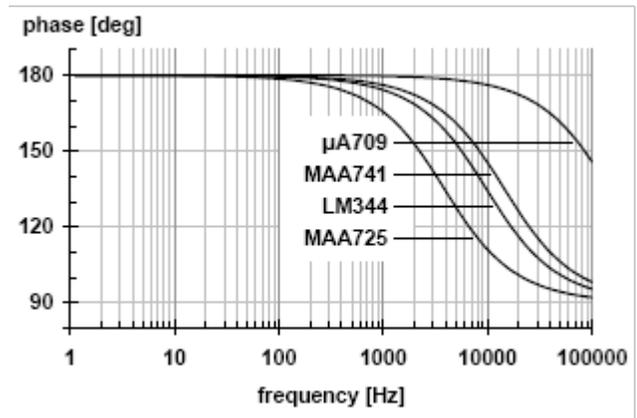
Fig. 13 phase response at  $R_0 = 10$  k $\Omega$
