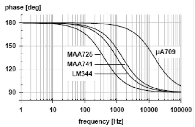
Fig. 15 phase response at  $R_0 = 1$  k $\Omega$
