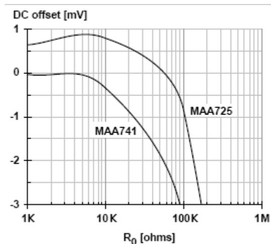
Fig. 21 detail of DC offset dependence on the value of  $R_0$  and the type of operational amplifier ( $R = 100 \text{ k}\Omega$ )
