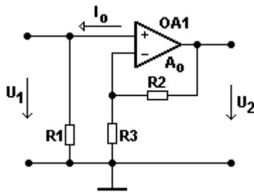
Fig. 1 non-inverting operational amplifier
