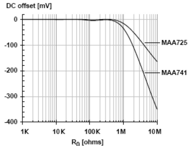
Fig. 20 DC offset dependence on the value of  $R_0$  and the type of operational amplifier ( $R = 100 \text{ k}\Omega$ )
