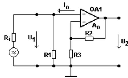
Fig. 2 non-inverting operational amplifier connected to the signal source
