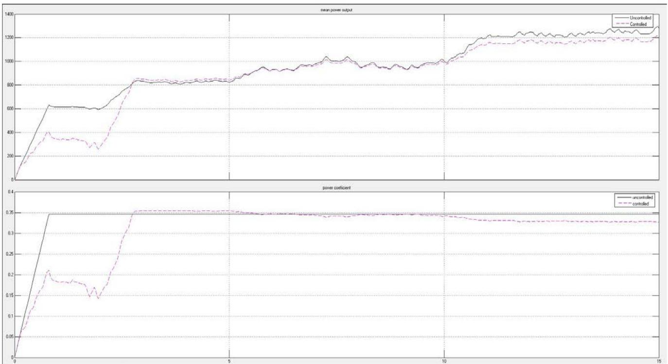
Fig. 6 effect of wind disturbances on output and power coefficient of 1KW turbine under uncontrolled as well as controlled operation with blade pitch angle as five degree
