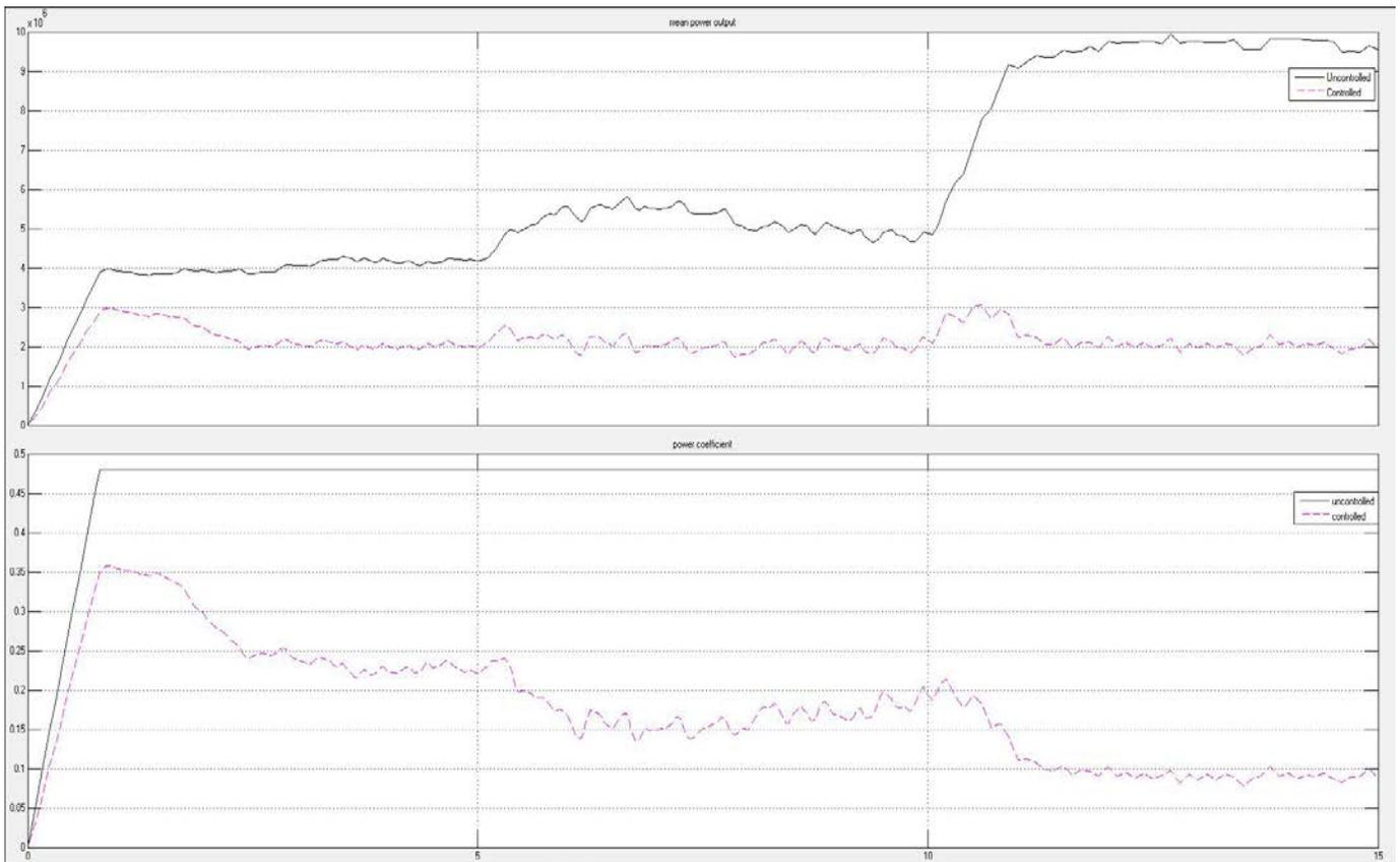
Fig. 8 effect of wind disturbances on output and power coefficient of 2MW turbine under uncontrolled as well as controlled operation with blade pitch angle as zero degree
