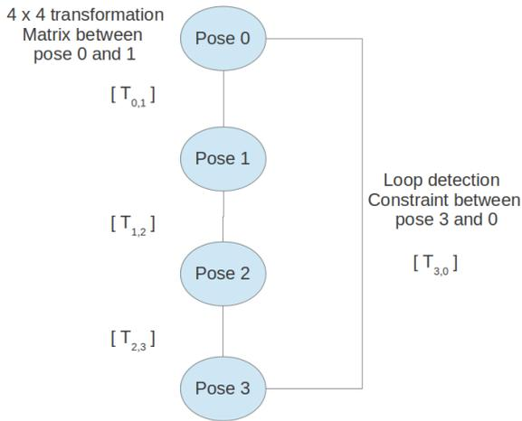
Fig. 3 An additional constraint is added to the graph.
