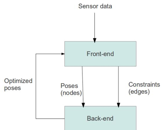
Fig. 1 The front-end and back-end of the SLAM process.
