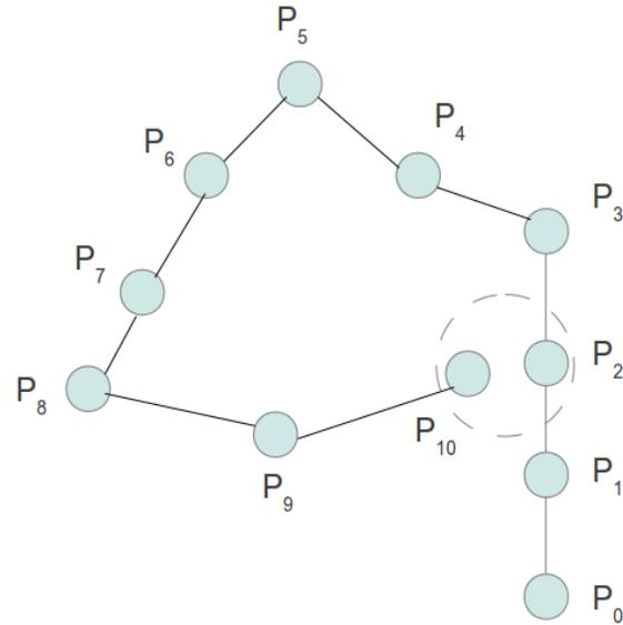
Fig. 4 Checking for closing a loop when reaching a node with a pose close to an existing one.
