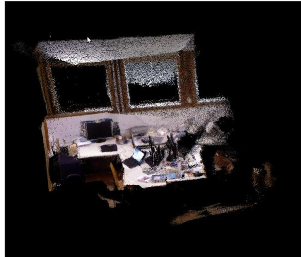
Fig. 8 The resulting map after processing the first 150 image sequence in the Freiburg1\_room dataset.
