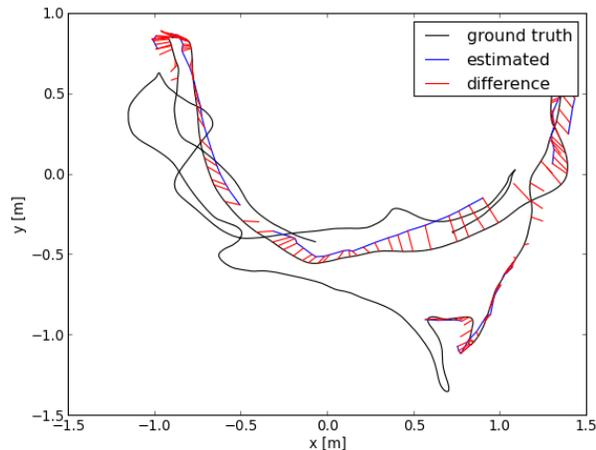
Fig. 9 The result trajectory compared to the groundtruth of the Freiburg1\_room dataset using  $g^2o$ .
