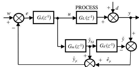
Fig. 1 Block diagram of a digital Smith Predictor
