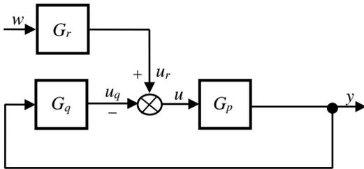
Fig. 2 Block diagram of a closed loop 2DOF control system
