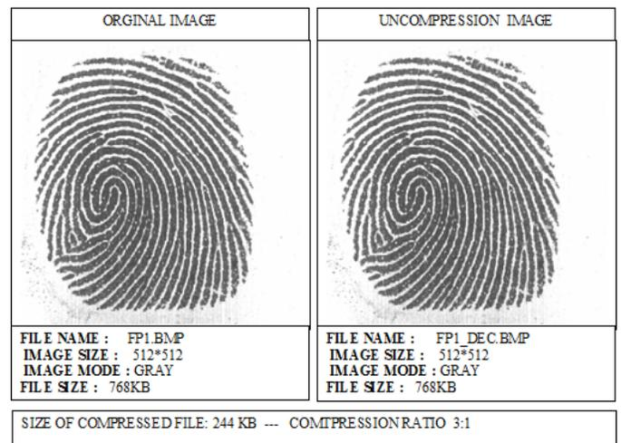
Figure 10. Fingerprints image compression details
