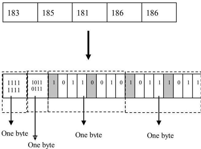
Figure 4. Example of encoded block of size 5x5
