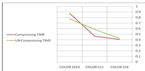
**Figure 12.** Average of compressing and Uncompressing Time for color images
