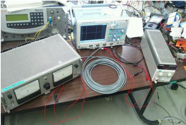
**Fig.5 Pulse generator using a single coaxial cable**
